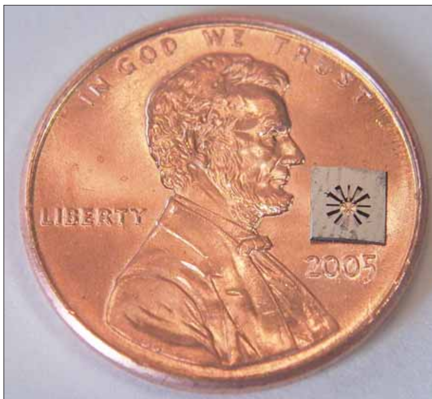
This mPhase ultra sensitive magnetometer used in cell phones and security applications is so small, it fits on the face of a penny.
